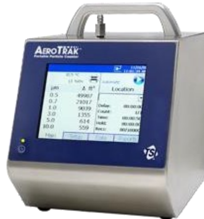
Figure 2: A velometer and method of measuring air velocity. Figure 3: Laser Particle Counter[9].
